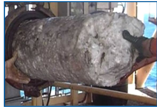
Gas hydrate blockages cost millions of dollars in lost production every year
